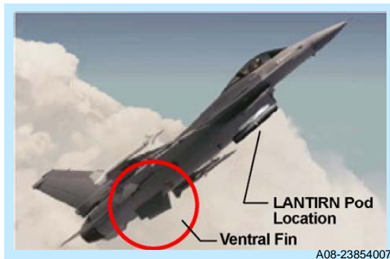
Figure 7 LANTIRN Pod Carriage on the F-16 (Ref. 24)
