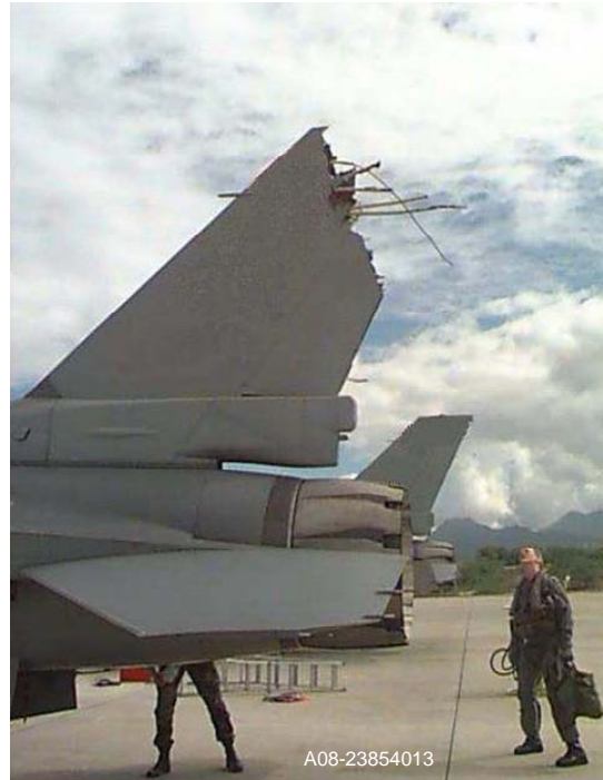
Figure 13 F-16 Vertical Fin Wake Turbulence Encounter (Ref. 17)
