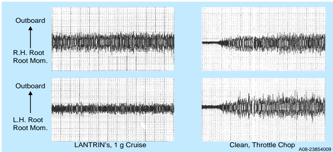
Figure 9 Ventral Fin Buffet Response to LANTIRN Pod Turbulence and Inlet spillage Turbulence (Ref. 24)
